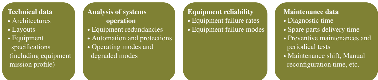
FIGURE 15.28 Reliability calculation taking into account ageing failures.
