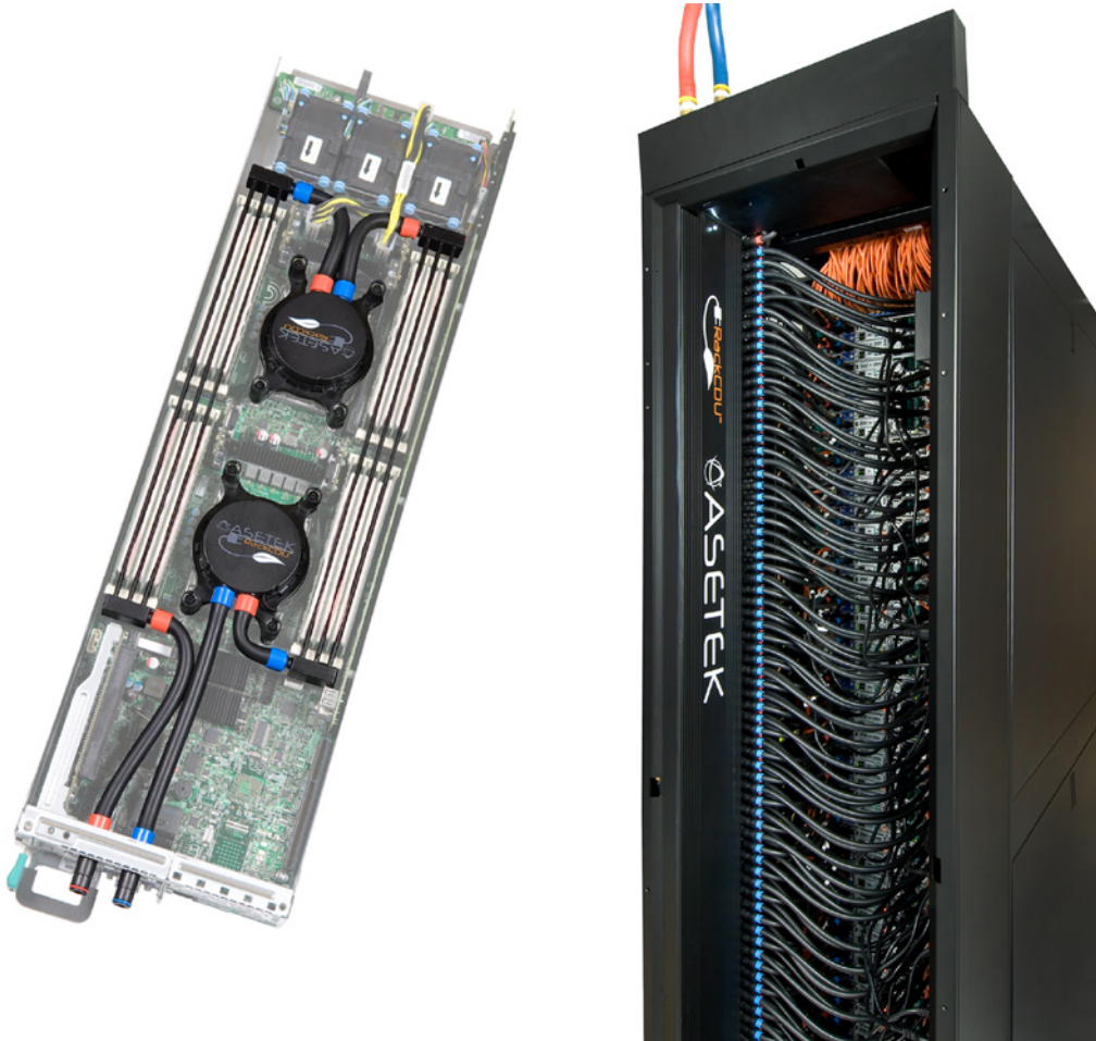
FIGURE 26.8 Intel memory cooled blade and rack CDU rear. Courtesy of Intel Corporation and Asetek Inc.
