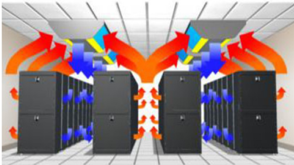
FIGURE 24.9 Overhead cooling unit solution. Courtesy of Schneider Electric.
